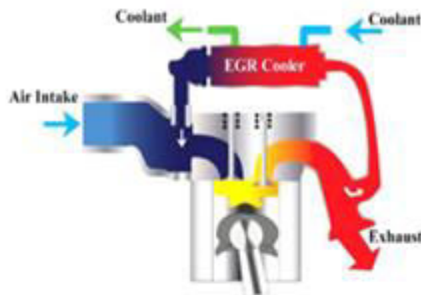
Fig.2 Operation of Exhaust Gas Recirculation System
