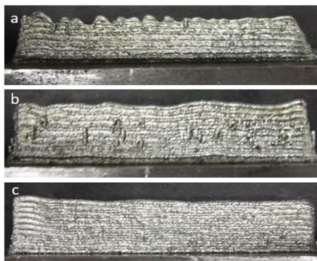
Figure 3: Seam build-up a) without control b) optimized initial conditions c) optimized parameters and initial conditions
