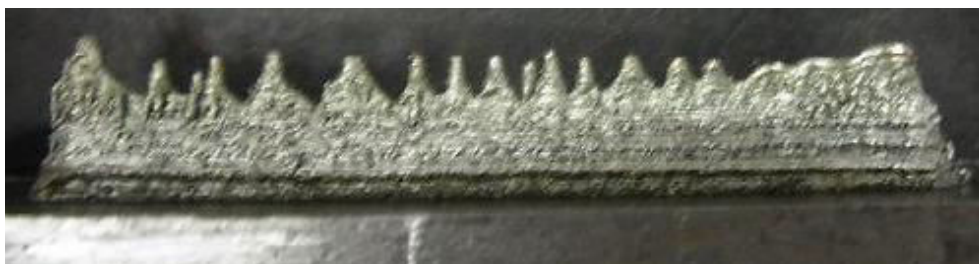
Figure 5: Influence of the working area on the structure build-up through LMD
